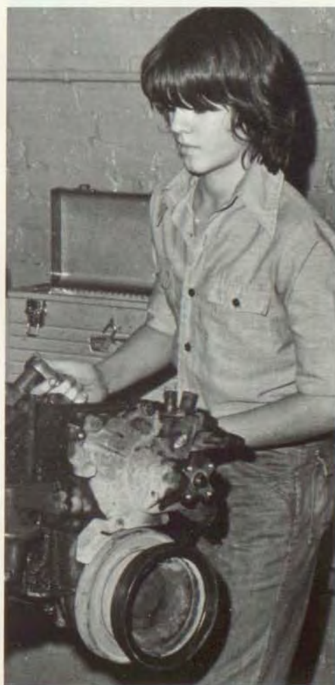
TO rebuild an engine Miles Latham uses a ridge-reamer to cut cylinder walls.
